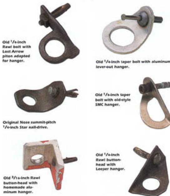
type bolts in coarse-grained rock (Joshua Tree, South Platte) or soft rock (Canyonlands) no matter what the diameter - are almost universally bad. Compression bolts can be easily removed with the standard procedure (see "Basic Replacement Technique," below); spinners can usually be pulled with the crowbar, skipping the piton step.
